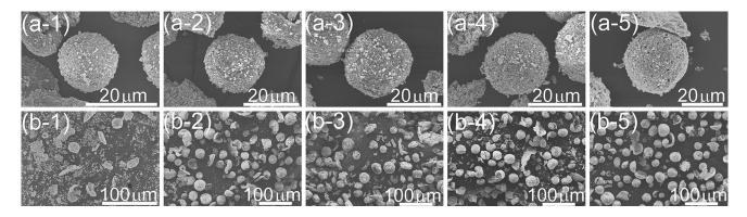
**Fig. 1** Typical SEM images showing the effect of spray power (a) and content of PVP in the starting suspension (b) on the sizes and the morphology of the hollow spheres, (a-1) net energy of 14 kW, (a-2) net energy of 20 kW, (a-3) net energy of 25 kW, (a-4) net energy of 30 kW, (a-5) net energy of 36 kW; (b-1) PVP content of 0.25%, (b-2) PVP content of 0.5%, (b-3) PVP content of 1.0%, (b-4) PVP content of 1.5%, (b-5) PVP content of 2.0%
