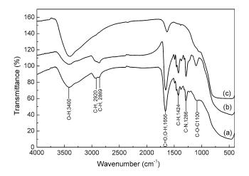
Fig. 5 FTIRs spectra of (a) the as-sprayed  $TiO_2$  hollow microspheres, (b) the as-sprayed  $TiO_2$ -Fe<sub>3</sub>O<sub>4</sub> hollow microspheres, and (c) the post-spray calcined  $TiO_2$ -Fe<sub>3</sub>O<sub>4</sub> hollow microspheres
