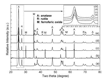
Fig. 3 XRD patterns of (a) the starting P25 nano powder, (b) the starting  $Fe_3O_4$  nano powder, (c) the as-sprayed  $TiO_2$  hollow spheres, (d) the post-spray calcined  $TiO_2$  hollow spheres, and (e) the  $TiO_2$ - $Fe_3O_4$  hollow microspheres
