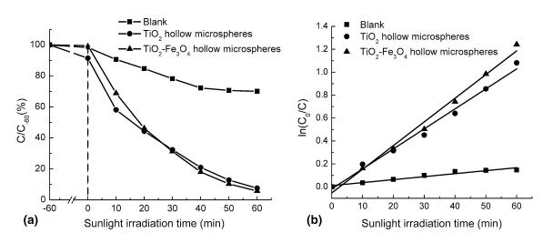
**Fig. 6** Photocatalytic activity assessment of the powder samples under sunlight irradiation, (a) variation of MB concentration vs. sunlight illumination time, and (b)  $\ln(C_0/C)$  against sunlight irradiation time in the presence or absence of the hollow microspheres
