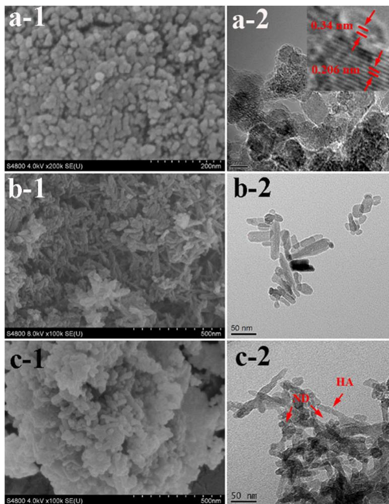
**Figure 1.** SEM (-1) and TEM (-2) images of the a) ND/BMP2, b) HA, and c) HA-ND/BMP2 composite powder. The inset in (a-2) is enlarged view of selected area.
