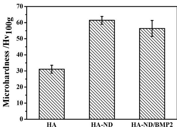
**Figure 5.** Vickers hardness of the coatings.
