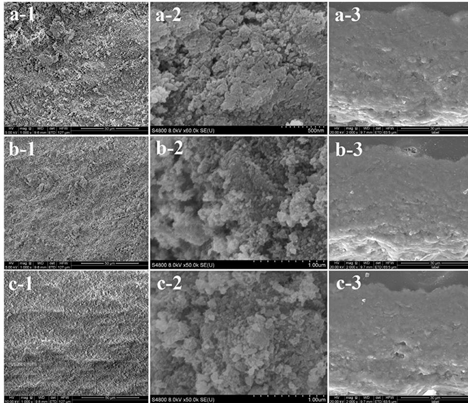
**Figure 2.** SEM images of the a) HA coating, b) HA-ND coating, and c) HA-ND/BMP2 coating. (-1: surface view, -2: enlarged view of selected area in -1, and -3: cross-sectional view).
