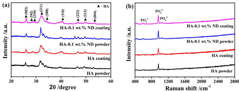
**Figure 3.** XRD patterns a) and Raman spectra b) of the powder and the coatings.
