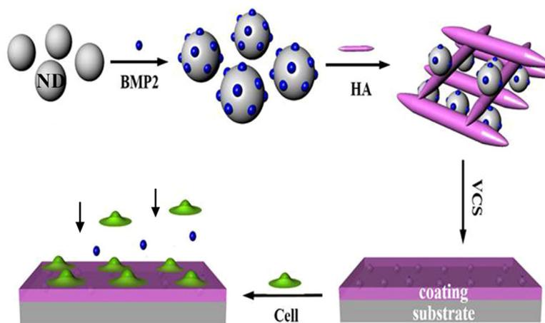
**Scheme 1.** Schematic illustration of the fabrication of the HA-ND/BMP2 powder and coatings.
