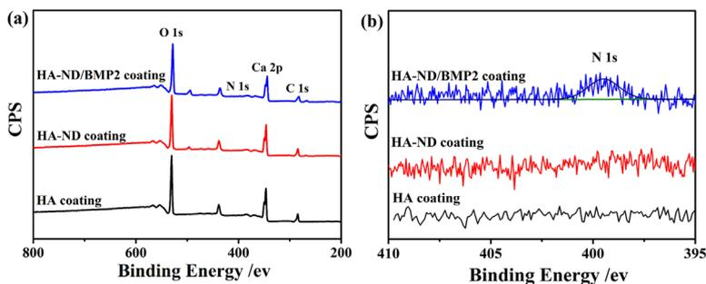
**Figure 4.** XPS spectra of the coatings a) and high resolution XPS spectra of N 1s b).
