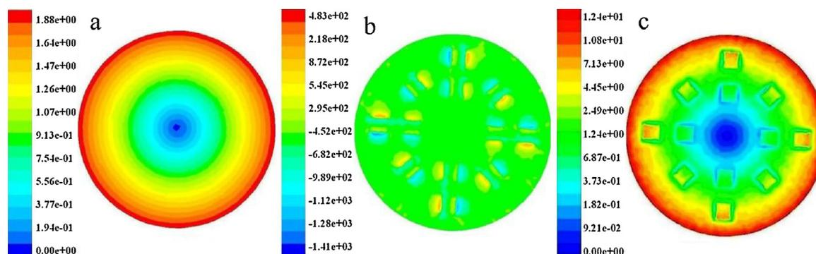
Fig. 2. Distribution of the flow velocity (a), flow pressure (b), and shear stress (c), the simulation was made with the rotation speed of 300 rpm.
