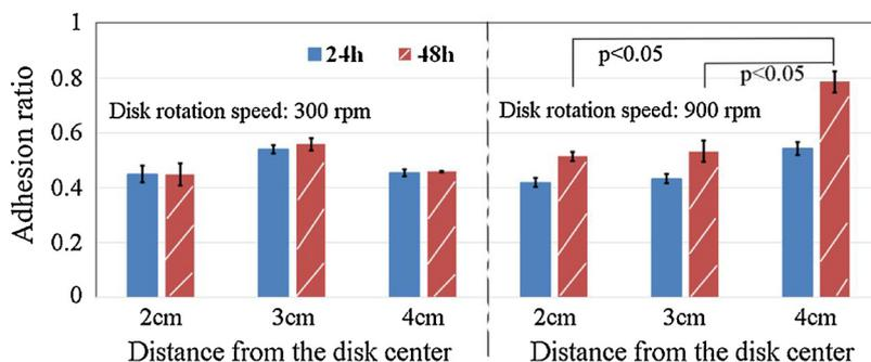
Fig. 4. Adhesion ratios of the bacteria on the stainless steel after 24 h and 48 h of exposure to the bacterial suspensions. The disk was rotated with the rotation speed of 300 rpm and 900 rpm.
