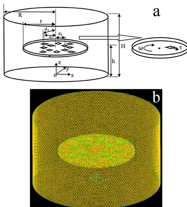
Fig. 1. (a) Schematic depiction of the geometry of the rotating system for generating turbulent flow, and (b) the unstructured mesh for the simulation.
