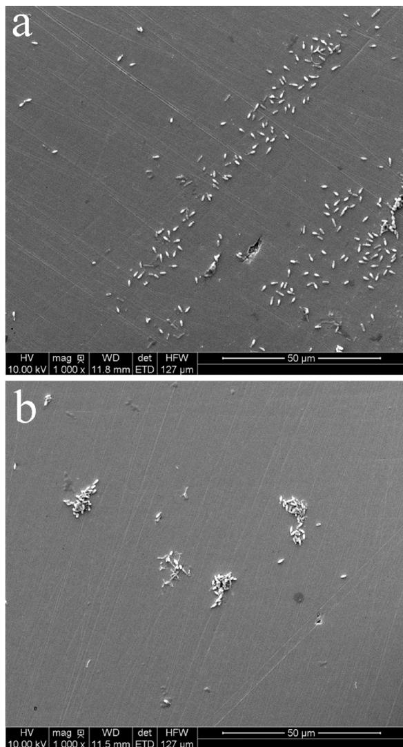
Fig. 6. SEM images of the *Bacillus* sp. biofilm formed on stainless steel after 1 week incubation with the rotation speed of 300 rpm (a) and 900 rpm (b).
