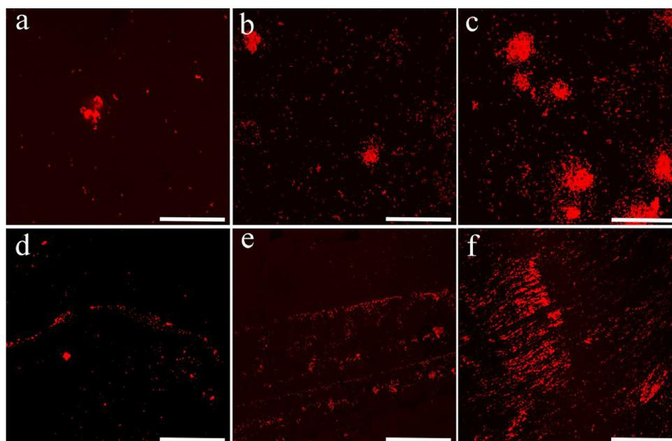
Fig. 5. CLSM images of the *Bacillus* sp. biofilm formed on the stainless steel after 1 week incubation. The rotation speed of the disk is 300 rpm (a: 2 cm, b: 3 cm, c: 4 cm, the length is the distance of the steel plate away from the disk center) and 900 rpm (d: 2 cm, e: 3 cm, f: 4 cm). The scale bar is 25 μm.
