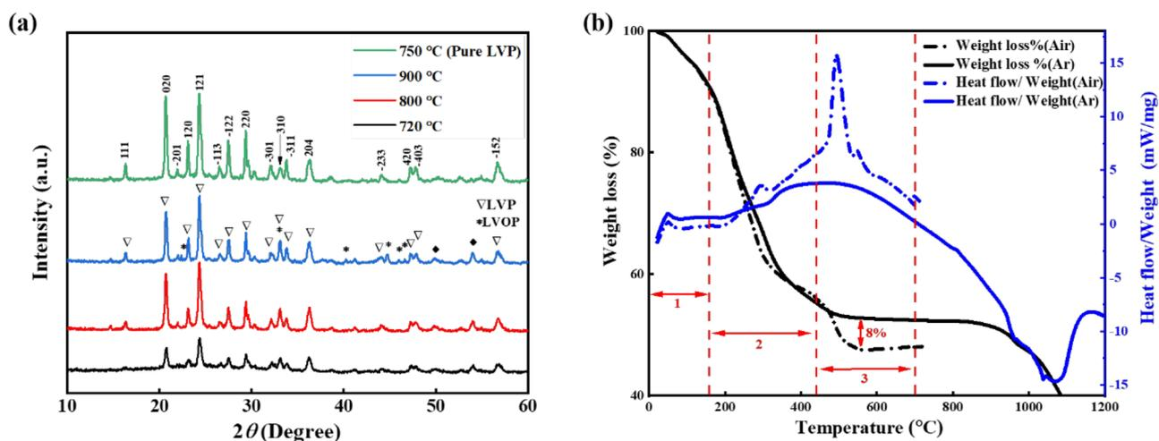
**Fig. 2** (a) XRD patterns of LVP-LVOP/C powder samples heated at 720 °C, 800 °C, 900 °C and pure phase sample (LVP/C-750 °C) (b) TGA and DTA curves of the (V-excess) as-synthesized sample in both air and argon atmosphere
