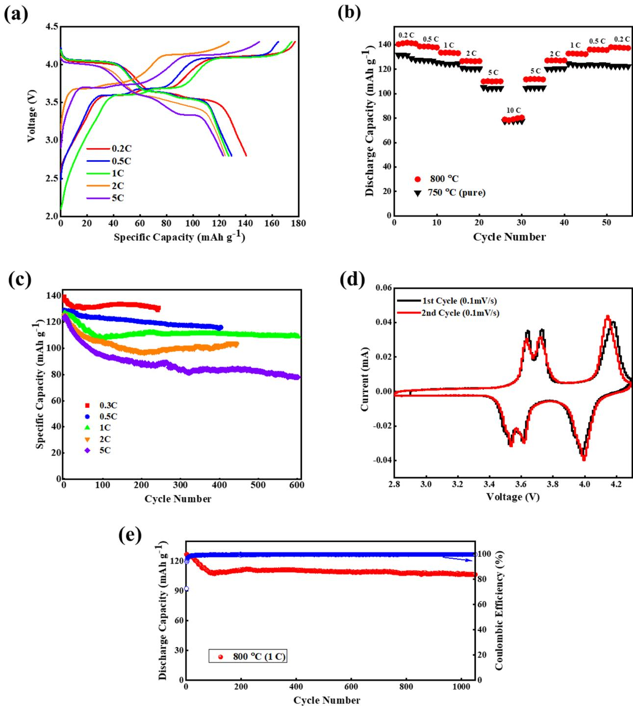
**Fig. 7** Initial charge/discharge curves at 0.2 C, 0.5 C, 1 C, 2 C, 5 C of LVP-LVOP/C-800 (a) comparison of rate capabilities of sample LVP-LVOP/C-800 with pure sample LVP/C-750 under different discharge rates (b) cycle performance; (c) at 0.3 C, 0.5 C, 1 C, 2 C; (d)
