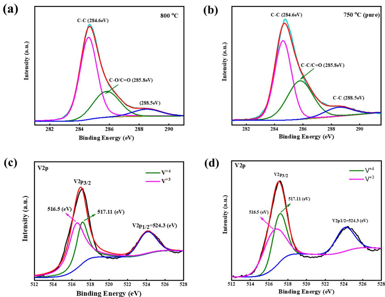
**Fig. 5** C1s and V2p XPS spectra and fitting results at (a) 800 °C (b) 750 °C (pure) and (c) 800 °C (d) 750 °C (pure), respectively
