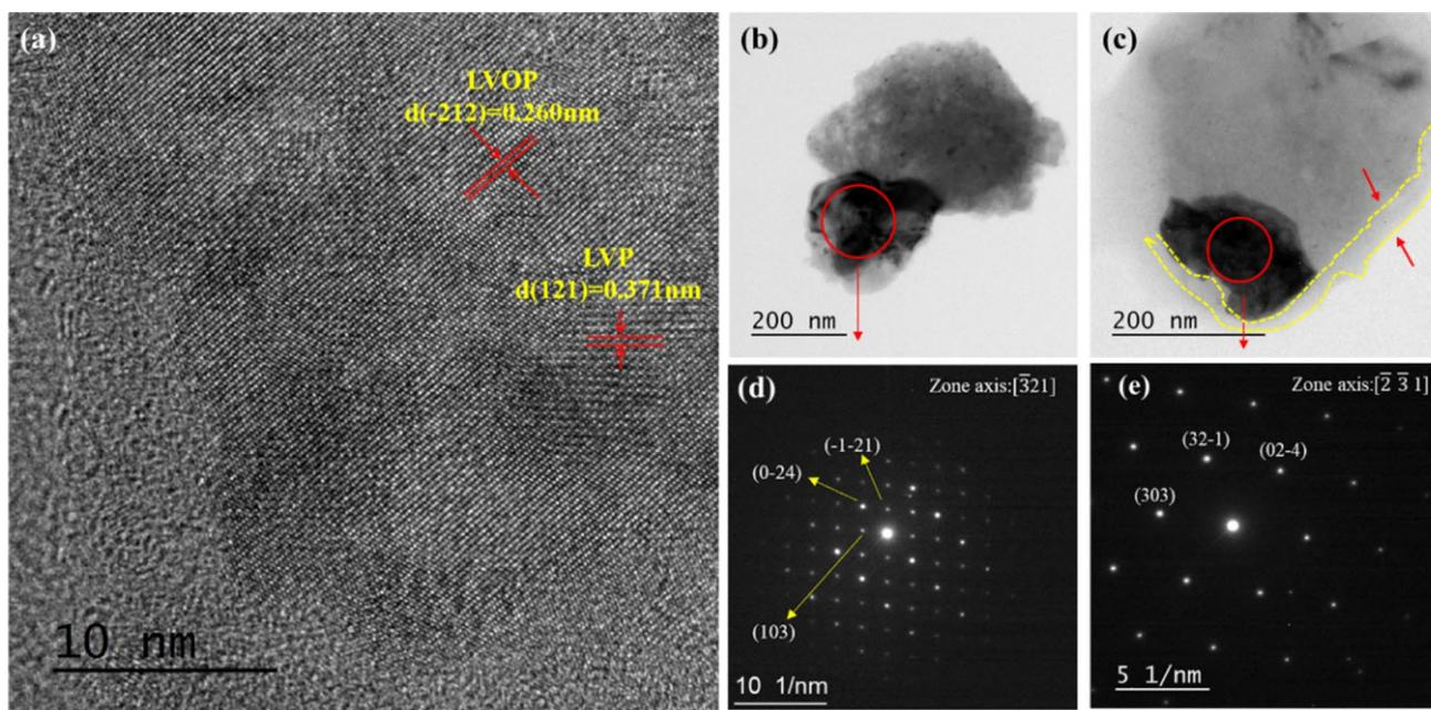
**Fig. 4** (a) HRTEM surface image; (d), (e) SAED patterns of area red circled in the image; (b), (c) LVP-LVOP/C powders sintered at  $800^\circ\text{C}$
