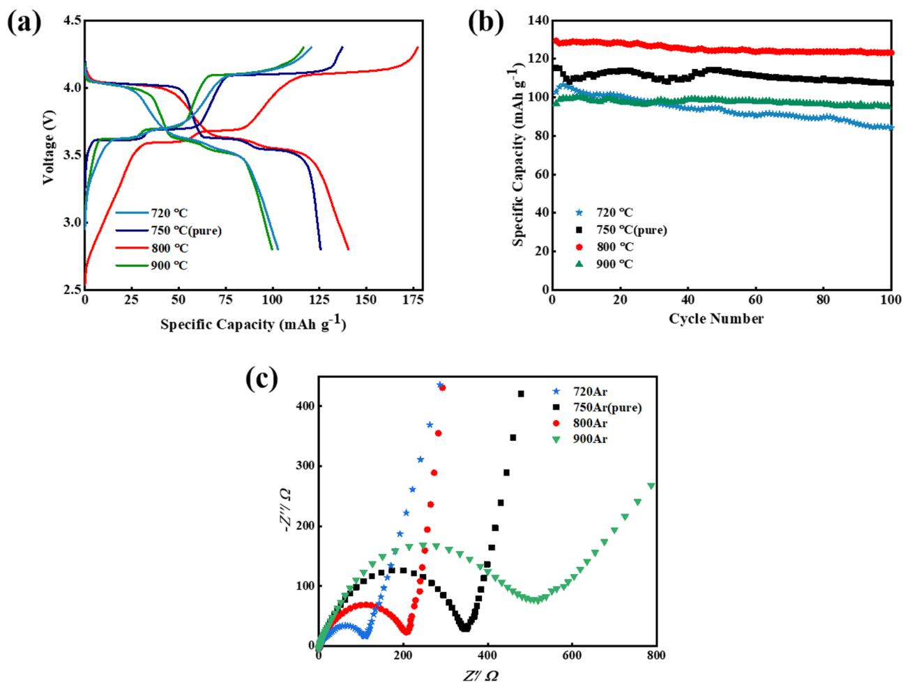
**Fig. 6** Comparison of initial charge and discharge curves at 0.2 C (a) cycle performance, (b) at 0.5 C, and (c) Nyquist plots of the LVP-LVOP/C and pure phase LVP/C-750 composite materials
